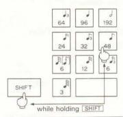
For example, to enter a step time of 48, hold [SHIFT] and press [6]().
