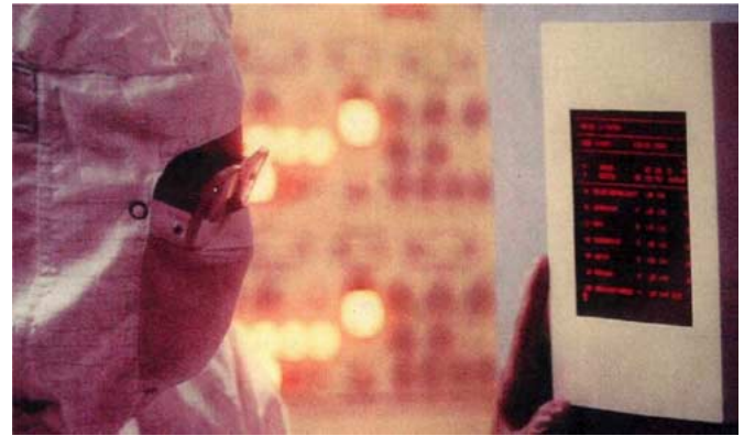
Fig. 19. First three electrode product introduced by AT&T in 1986 [31], [32]. This monochrome surface-discharge panel had the data electrodes on the front plate in addition to the parallel sustain electrodes on the back plate. The barrier ribs were on the front between the data electrodes. All of today's color products use a similar three electrode structure except that the roles of the front plate and the back plates are exchanged. Property of AT&T archives. Reprinted with permission of AT&T.
