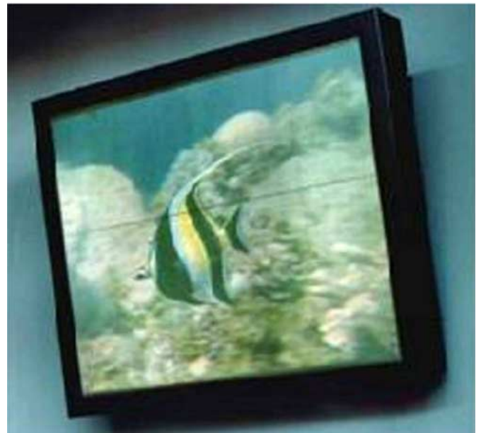
Fig. 22. The 31-in prototype developed by Fujitsu in 1990. This prototype had all the elements of the modern color plasma display TV: three-electrode structure with phosphor on the back plate [35], ADS grayscale [37] and Ne–Xe gas.
