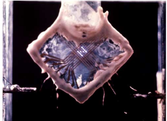
Fig. 4. Early 4 \times 4 pixel panel presented in the first publication of the plasma display panel by University of Illinois at 1966 Fall Joint Computer Conference [10]. This panel was the first to have more than one pixel. It was also the first to achieve matrix addressability [11], [12].
