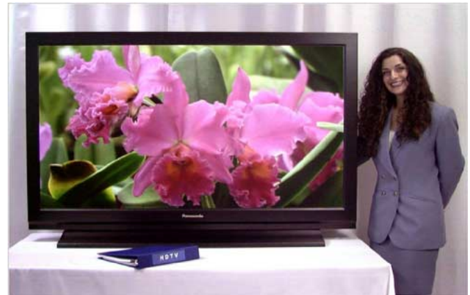
Fig. 26. HDTV 60-in diagonal prototype developed by Plasmaco in 1999 [41]. This demonstrated that large screen HDTV could be very attractive. Today we have 71-in products and the largest prototype is 102 in.
