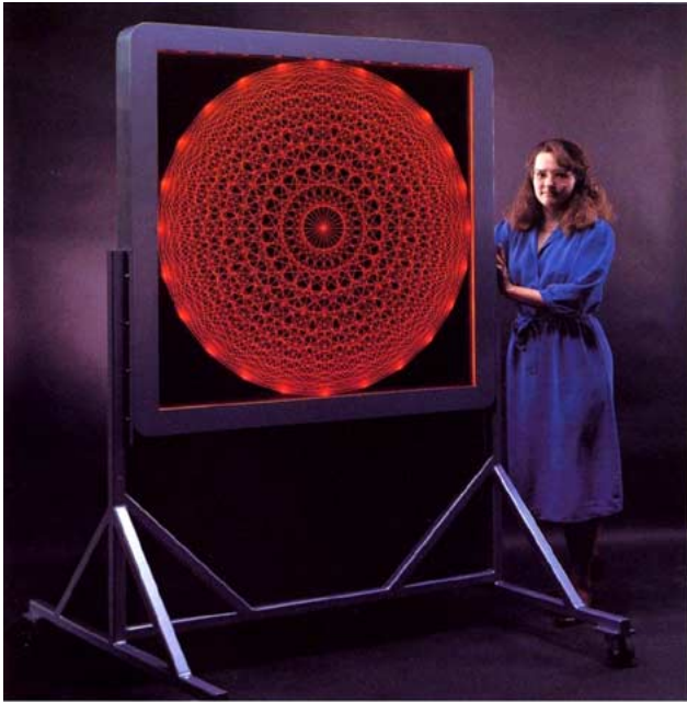
Fig. 17. The 59-in diagonal product with 2048 \times 2048 monochrome pixels developed by Photonics in 1987 [29]. This product clearly demonstrated that large size plasma displays were possible. This presented good proof that the issues of electrode resistance, inductance, panel capacitance, and addressability of such large panels were manageable.
